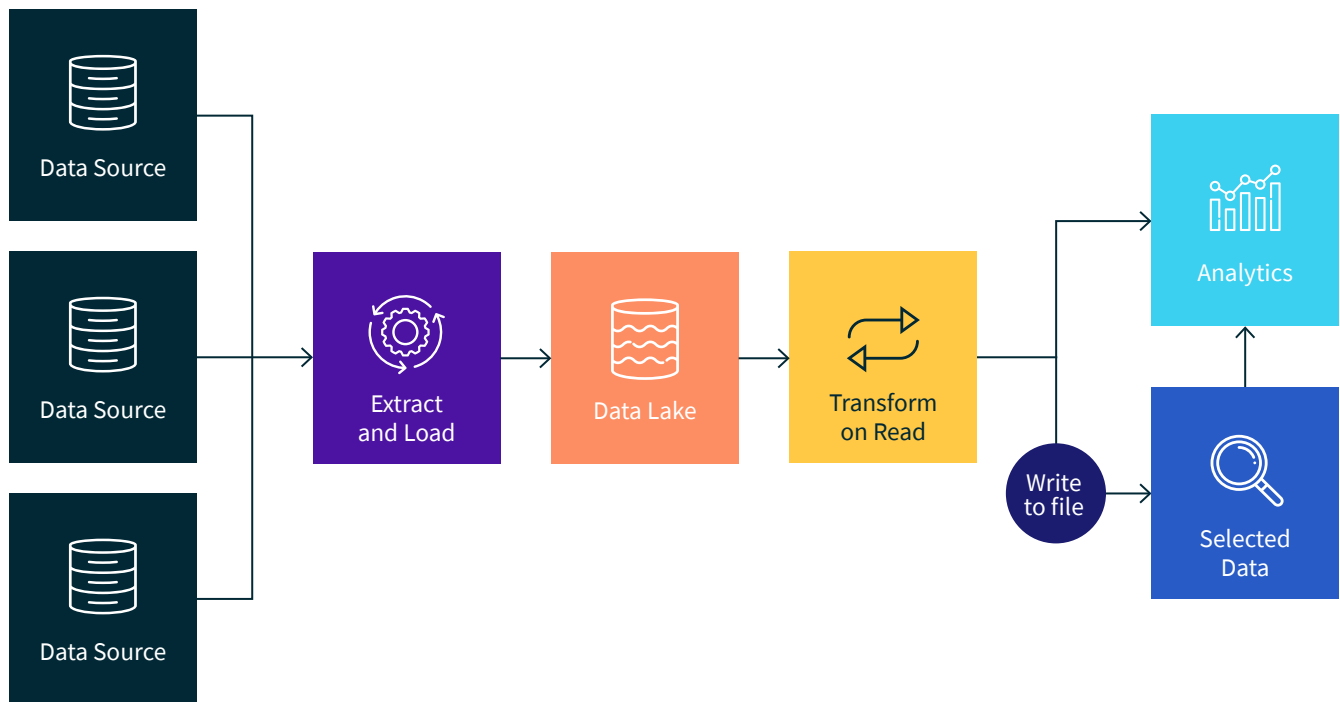
Figure 3. ELT Process – Transformation Occurs When Data Is Read
